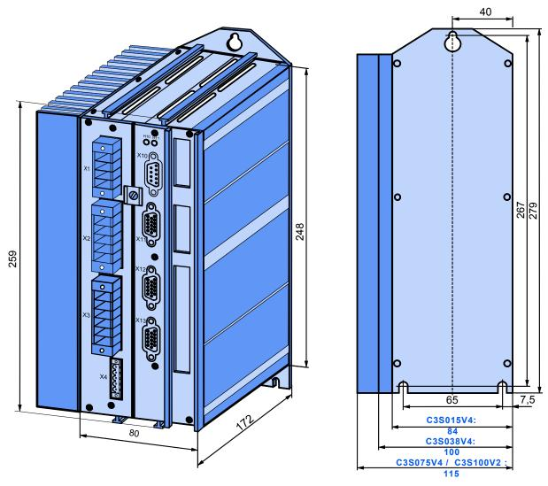
Please respect an appropriate mounting gap in order to ensure sufficient convection:
