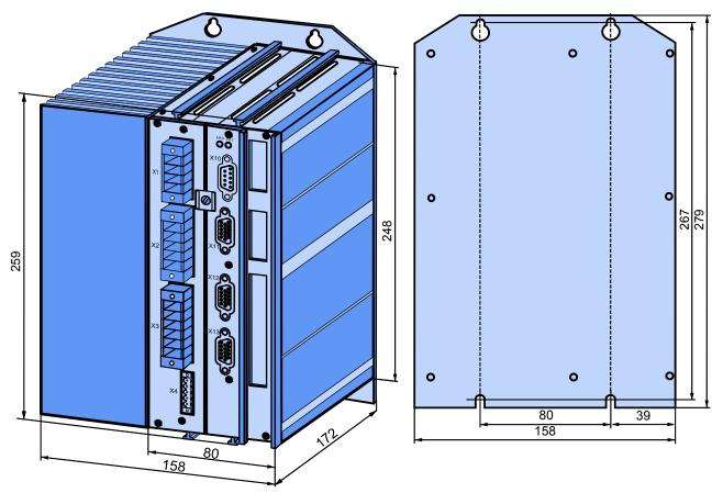
Please respect an appropriate mounting gap in order to ensure sufficient convection:
