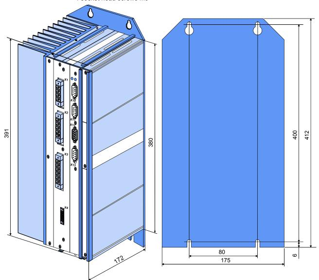
Please respect an appropriate mounting gap in order to ensure sufficient convection:
