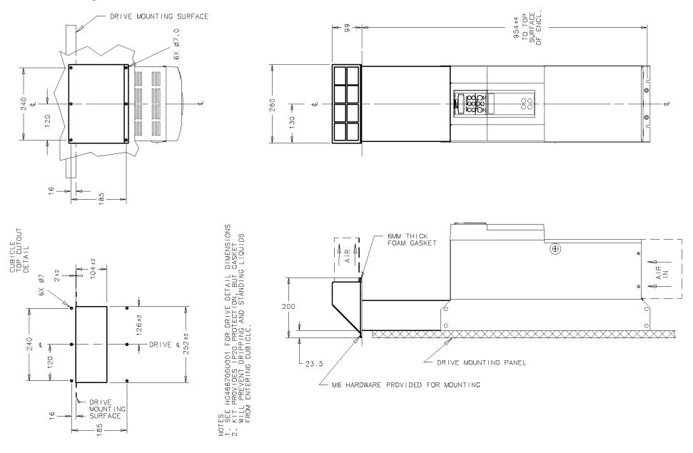
Figure 3- 33 Frame 4: 380-830A External Vent Kit Installation – Drg No. HG466700U002
