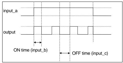
Creates a pulsed FALSE / TRUE output of programmable frequency.
