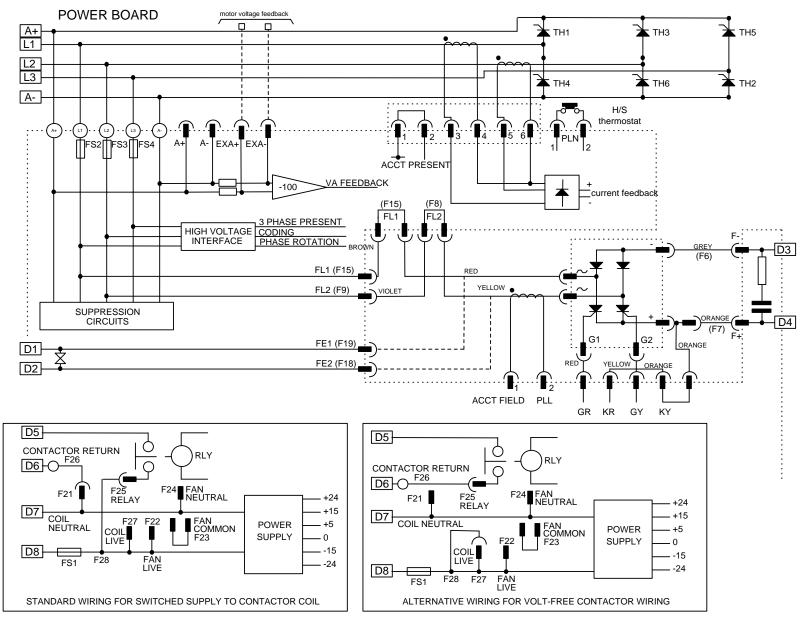
Figure 3-19 2 Quad Power Circuit - using AH385851U003, U004 (Frame 3)
