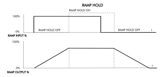
The ramp will function when a ramp input is present. When DIGIN 2 (C7) is ON, RAMP HOLD stops the ramp from changing. Even when the ramp input signal is removed, RAMP HOLD keeps the ramp output from changing. Once RAMP HOLD is OFF, the ramp resumes.
