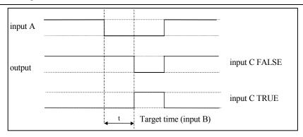
A programmable delay between receiving and outputting a Boolean FALSE signal.
