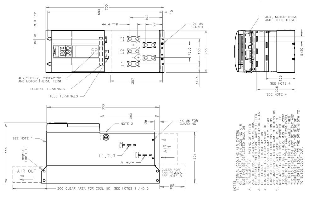
Figure 3- 32 Frame 4: 380-830A Stack Assembly – Drg. No. HG466700U001
