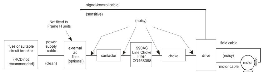
Figure 3-5 Cabling Requirements
