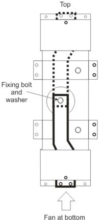
Fan at bottom of phase assembly
