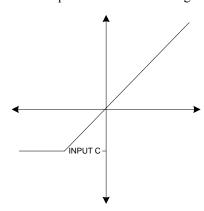
Action of clamp when INPUT C is negative or zero
