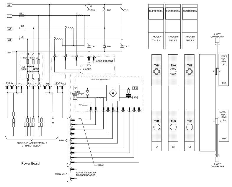
Figure 3- 25 2 Quad Power Circuit – Frame 6 & Frame H Units using AH466001U001
