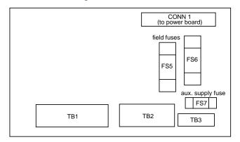
Figure 3-14 Terminal Board - AH466407
