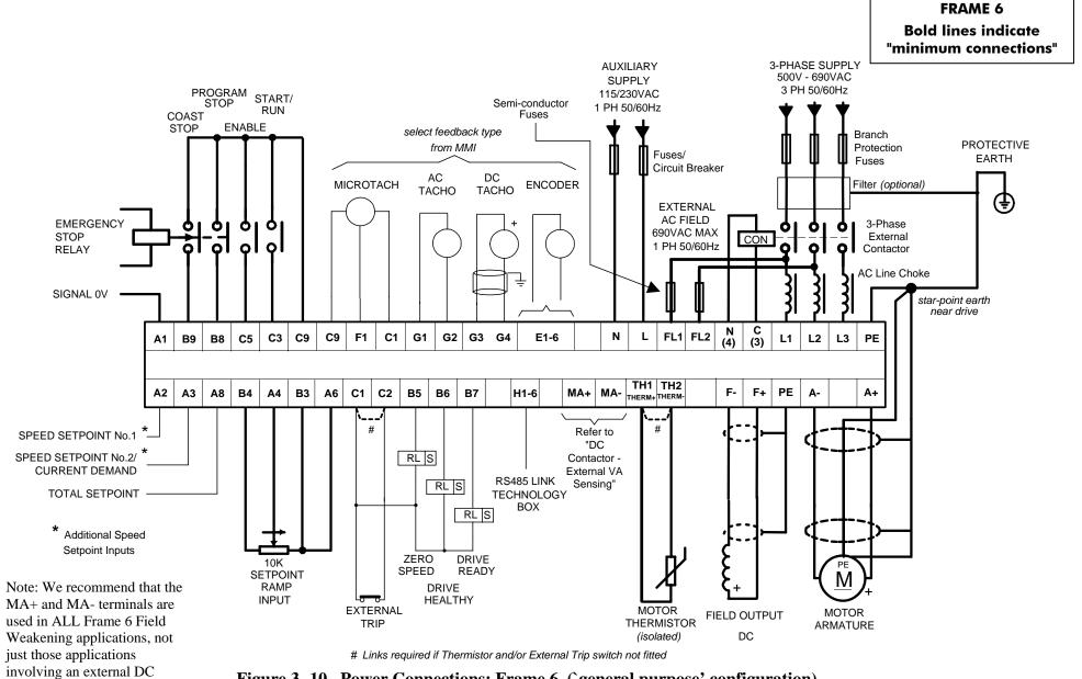
Figure 3-10 Power Connections: Frame 6 ('general purpose' configuration)
