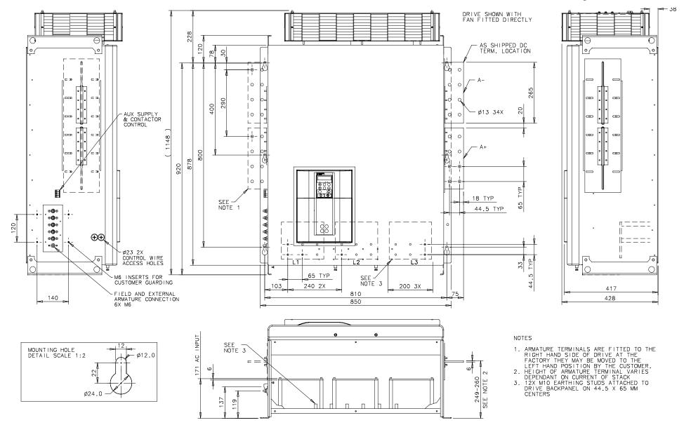
Figure 3- 38 Frame H: 1200A-2700A Stack Assembly (Non-regenerative) - Drg No. HG466433U000/1
