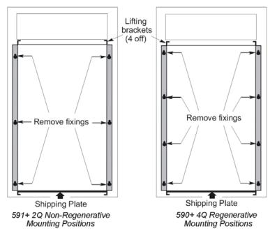
Figure 3-1 Lifting Details (Frame H)
