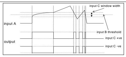
This function outputs TRUE when INPUT A is within a programmable range, and FALSE otherwise.
