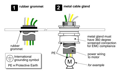
Figure 3-6 Cable and Screen Fixings
