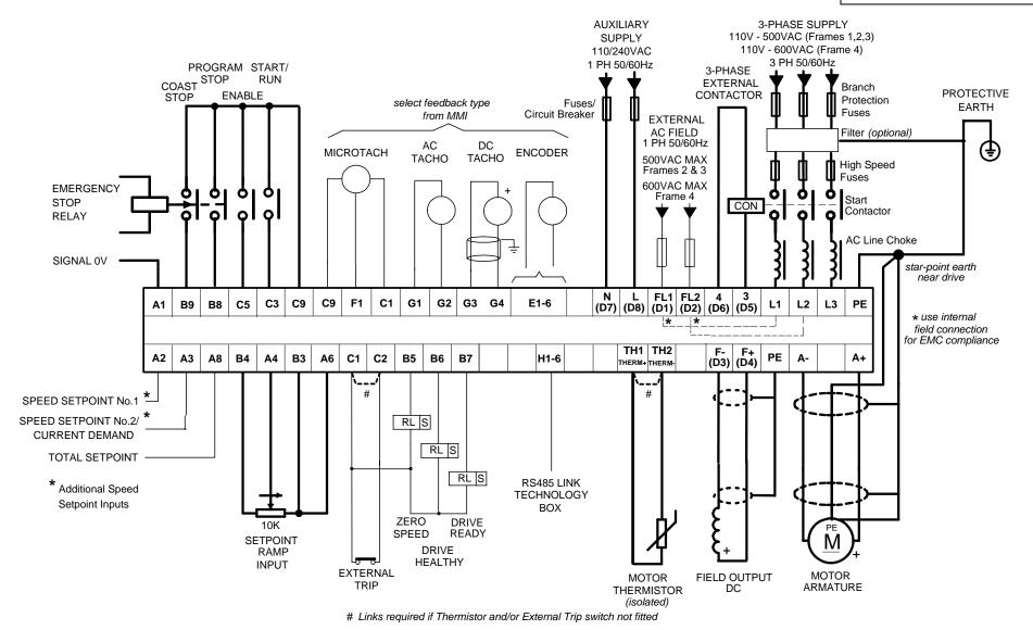
Figure 3-8 Power Connections: Frames 1, 2, 3 & 4 (general purpose configuration)
