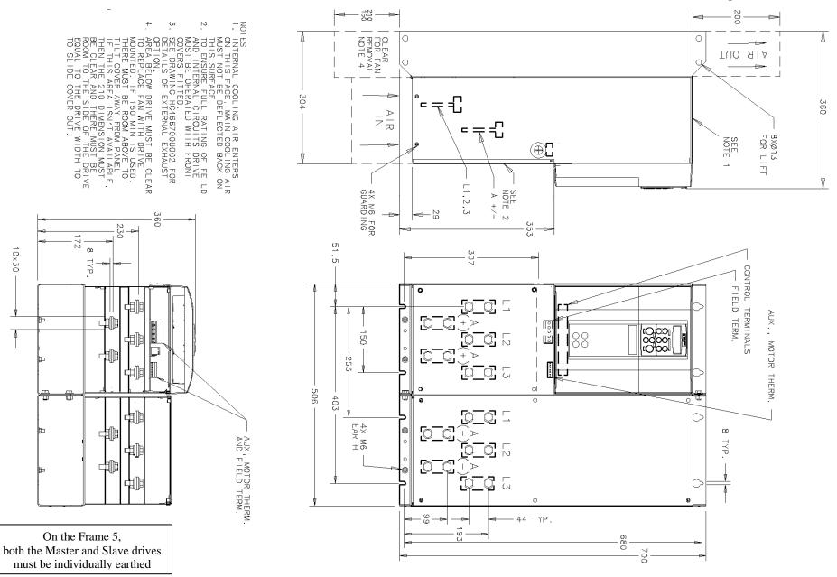
Figure 3- 34 Frame 5: 1580A Stack Assembly – Drg No. HG466700U110
