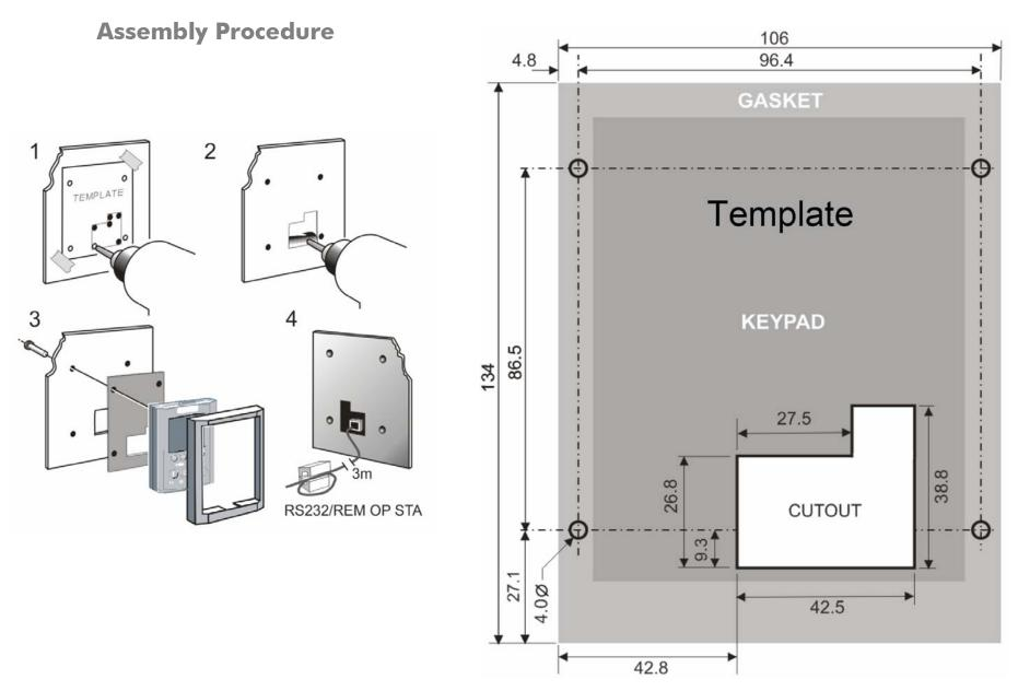
Figure 3-27 Mounting Dimensions for the Remote-Mounted Keypad
