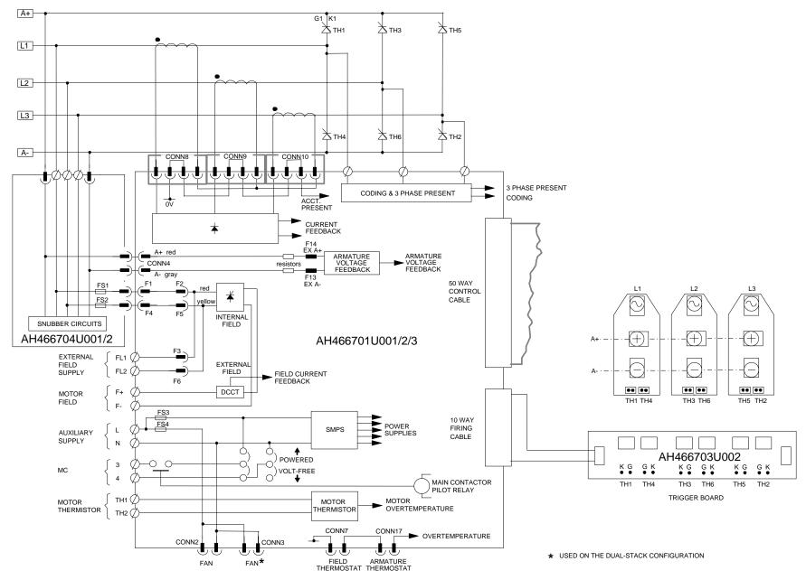
Figure 3- 24 2 Quad Power Circuit – Frame 4 & 5 Units using AH466701
