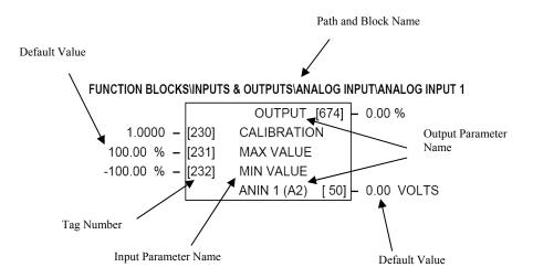
**Figure D-3 Function Block Parameter Information**
