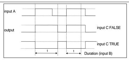
Creates an output of adjustable minimum time when INPUT A is TRUE. (INPUT A is assumed to be a sequence of TRUE pulses and FALSE off periods.)
