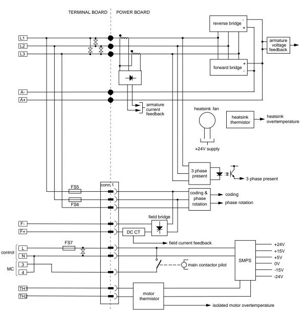
Figure 3- 15 Connection Diagram for Power Board and Terminal Board - AH470280 (Frame 1)
