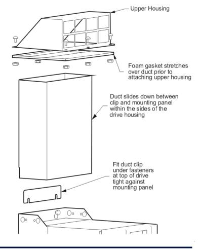
Figure 3-3 Frames 4 & 5 External Vent Kit
