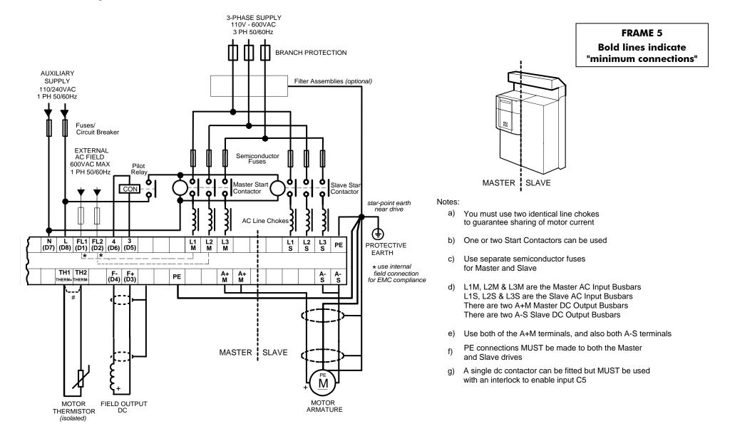
Figure 3-9 Power Connections: Frame 5 ('general purpose' configuration)
