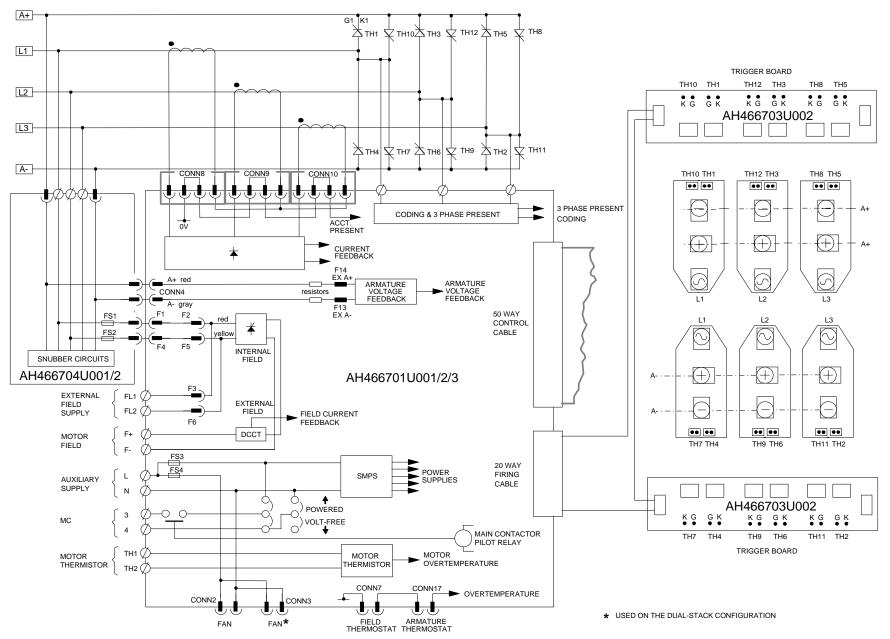
Figure 3- 23 4 Quad Power Circuit – Frame 4 & 5 Units using AH466701
