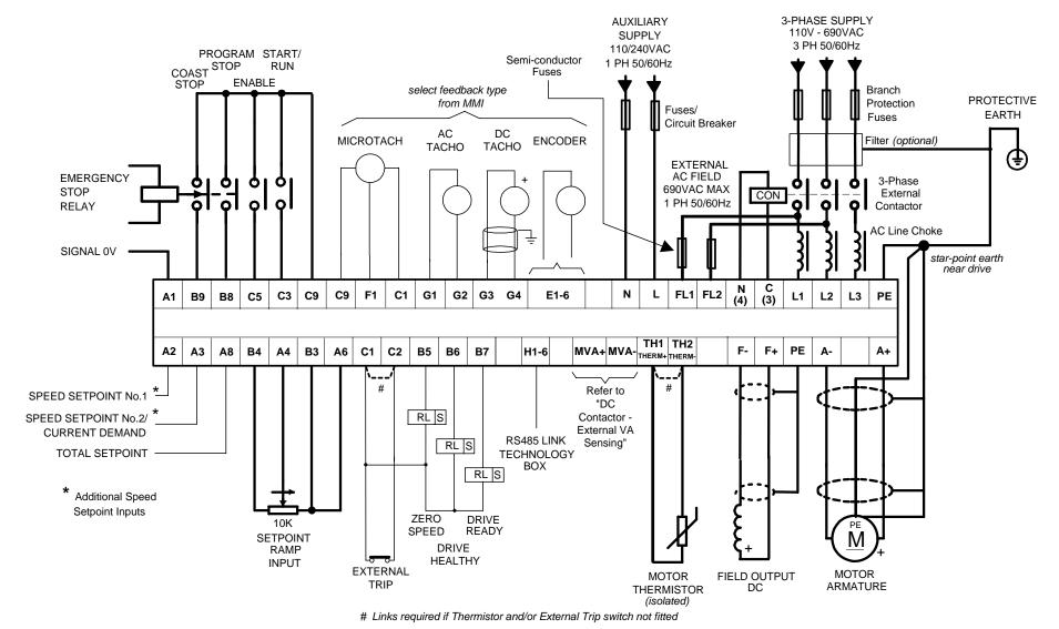
Figure 3-11 Power Connections: Frame H ('general purpose' configuration)
