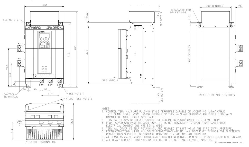
Figure 3-31 Frame 3: 270A Stack Assembly - Drg No. HG466428
