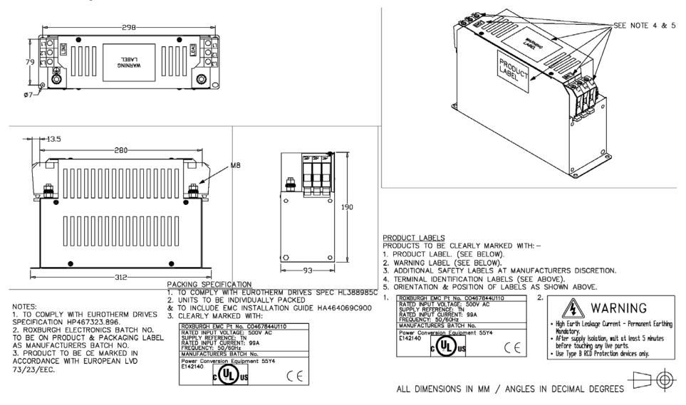
Figure 3-43 Filter Mounting Details, Part No. CO467844U110 for 590+ Frame 2:110 Amp
