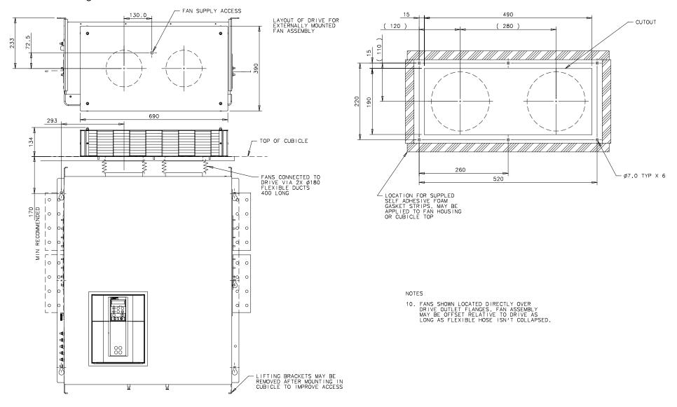
Figure 3- 39 Frame H: 1200A-2700A Stack Assembly (Non-regenerative) - Drg No. HG466433U000/2
