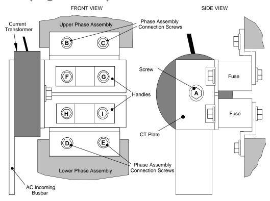
Figure 8-1 590+ (Frame H) Fuse Replacement Diagram
