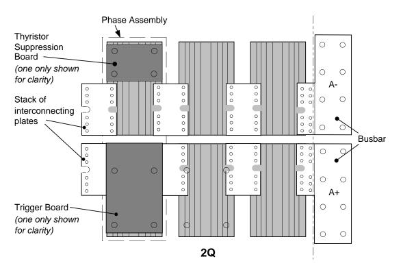
Figure 8-3 Front View of Phase Assemblies
