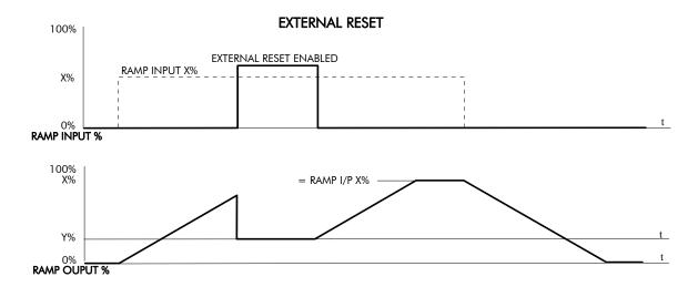
The ramp input is set to X% at time  $t_0$ . The ramp output will increase at the ramp rate. While EXTERNAL RESET is ENABLED, the ramp output resets to RESET VALUE (Y%). When EXTERNAL RESET is DISABLED, the ramp output continues to follow the input signal.
