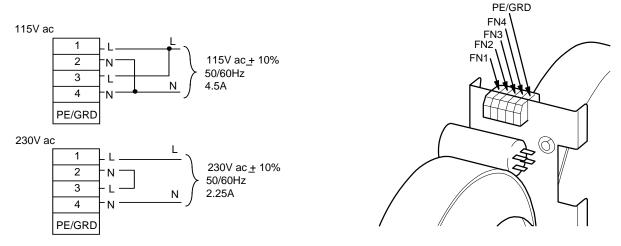
Figure 3-2 Frame H Fan Wiring Diagram
