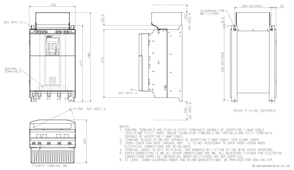
Figure 3- 30 Frame 3: 180A Stack Assembly - Drg No. HG466427
