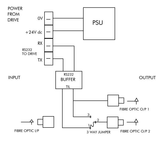
Figure A-2 Wiring Diagram for 5703/1 Speed Repeater
