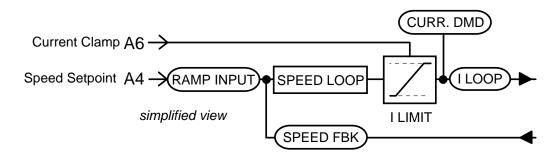
In both cases, the Current Limit is controlled via terminal A6 (ANIN5).
