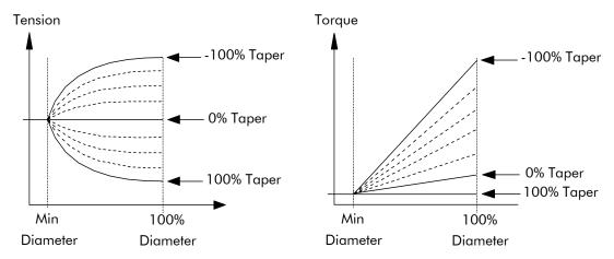
The result is multiplied by TENSION SPT. to get TAPER DEMAND. When the taper setpoint is at 100%, the motor produces constant torque. That is, a constant torque from core to full roll, and the tension falls off as the roll builds.
