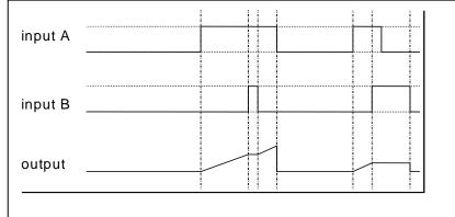
Times the period elapsed from when INPUT A is set TRUE and held TRUE, to when INPUT B becomes TRUE.
