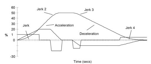
Example acceleration graph for a velocity 60 %/s maximum Acceleration of 20 %/s² and a jerk of 10 %/s³
