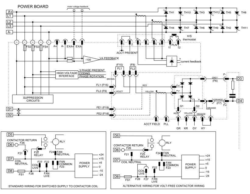
Figure 3- 21 4 Quad Power Circuit - using AH385851U002, U005 (Frame 3)
