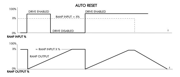
When AUTO RESET is ENABLED, ramp output resets to RESET VALUE each time the drive is enabled. In this example RESET VALUE is 0.00%. It does not reset if the drive is disabled.
